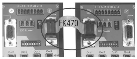
Cascading lines use the same common GND potential as the power supply of the unit. This however does not mean any disadvantage in terms of galvanic isolation etc. since cascading units are always mounted alongside and are also supplied from the same power source.
