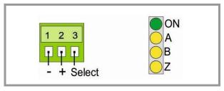
The upper LED (green) signals that power is applied to the unit.
