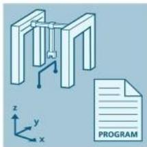
Using the "LAxesGrpCtrl" block library for controllers in the SIMATIC S7-1200 family, it is possible to coordinate and traverse multiple axes of a Cartesian handling system on a predefined motion path as a synchronous point-to-point (sPTP) movement in space.
