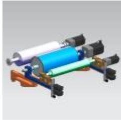
This application example allows you to simulate SIMATIC Print Standard Add-On Cylinder Positioning using PLCSIM Advanced, SIMIT and NX Mechatronics Concept Designer (MCD).
