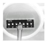
Any dosage required can be set via DIP switch combinations
