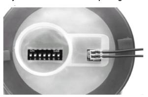
Setting same as so far. Extend contact cable and connect to limit switch or contactor with floating contact. No external power supply required.
