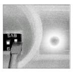
Make DIP switch 7 active. Green LED blinks flashes. Red LED flashes repeatedly 15 times.
