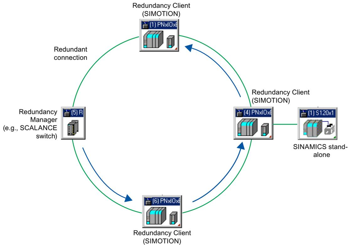
Figure 5-26 Ring topology for media redundancy without fault
