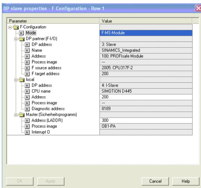
Figure 9-45 Master-slave coupling in PROFIsafe
