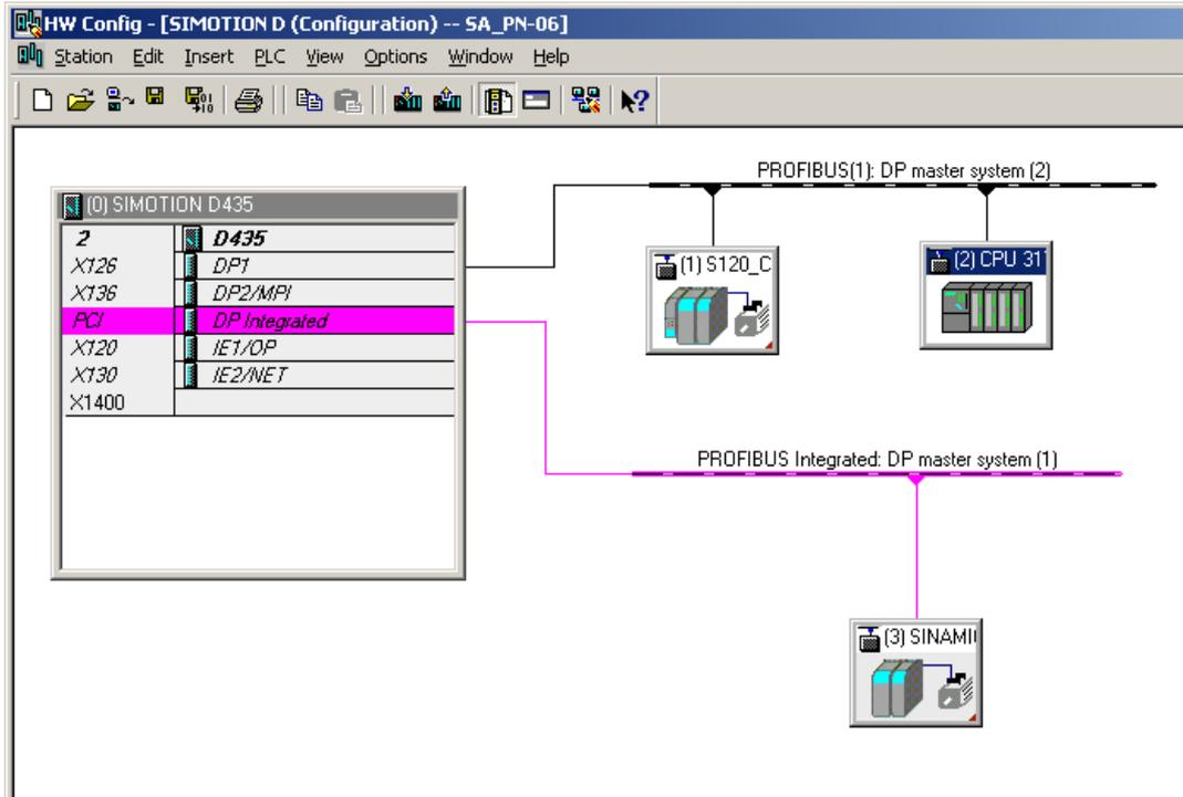
Figure 9-52 HW Config failsafe data exchange broadcast
