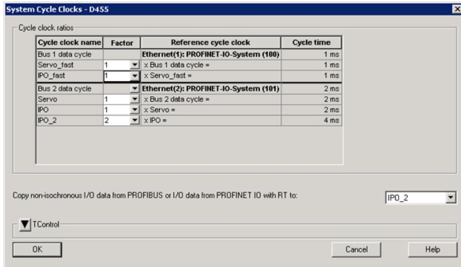
Figure 5-46 Servo and Servo\_fast system cycle clocks
