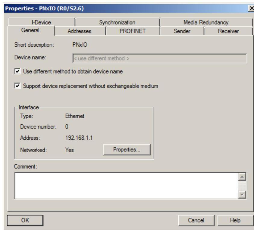
Figure 5-54 Obtaining the device name using a different method
