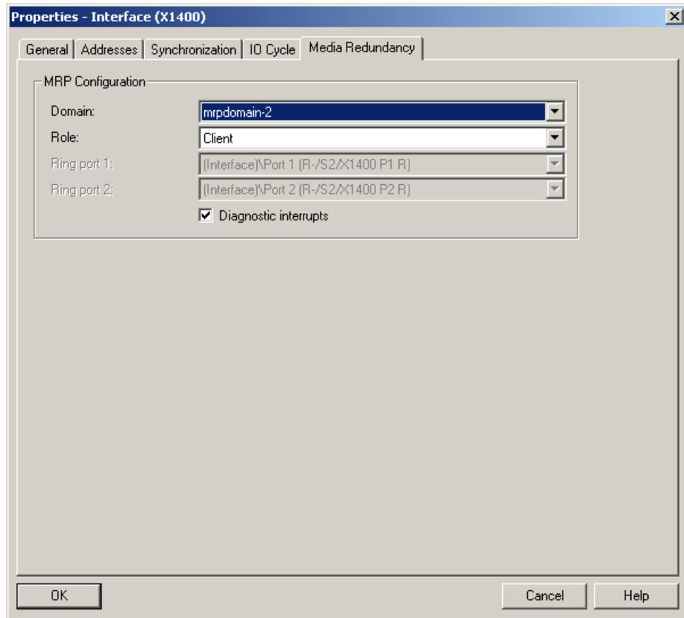
Figure 5-61 Properties of redundancy client
