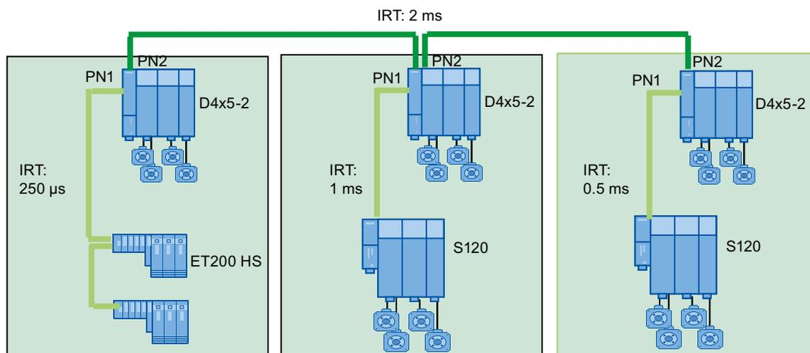
Figure 5-19 Application 3 for two PROFINET IO interfaces
