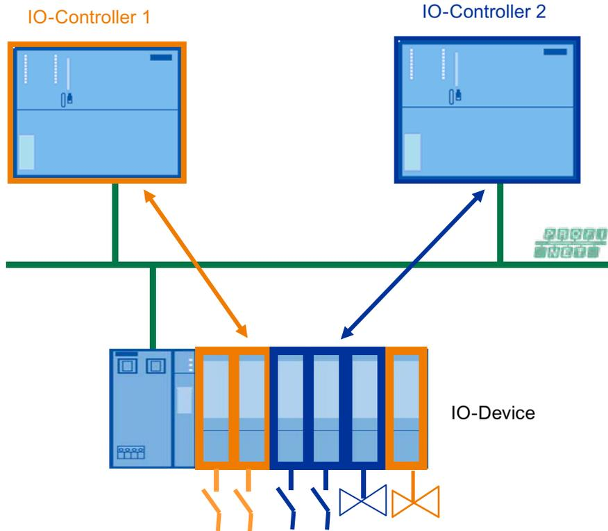
Figure 9-26 Schematic diagram of Shared Device
