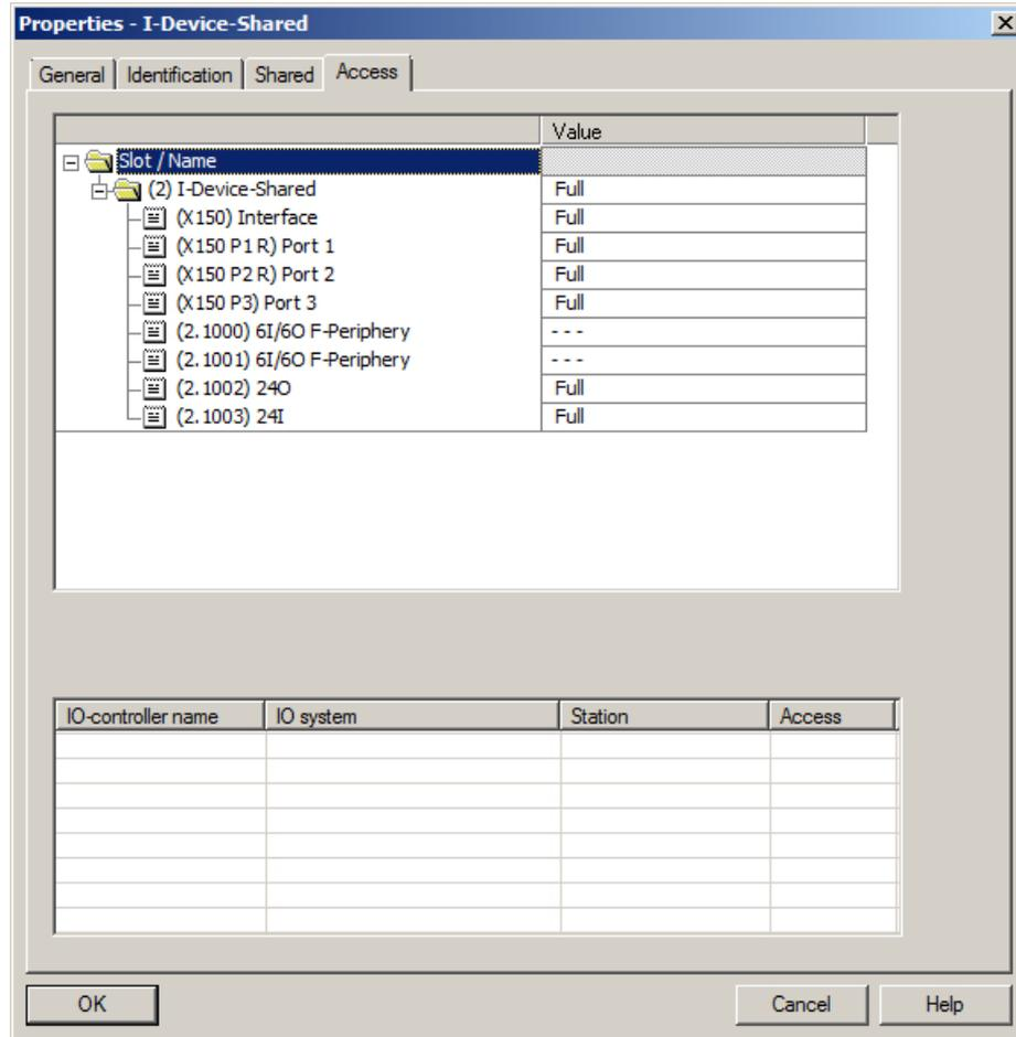
Figure 9-38 Setting access to the submodules for the SIMOTION D
