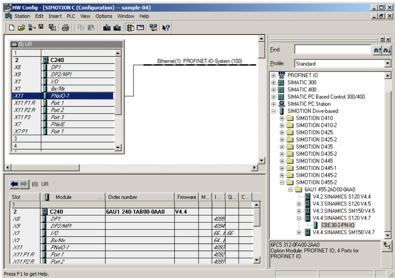
Figure 5-41 HW Config with PROFINET for C240 PN
