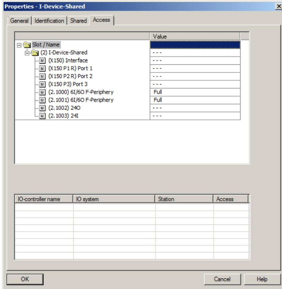
Figure 9-36 Setting access to the submodules for the F-CPU
