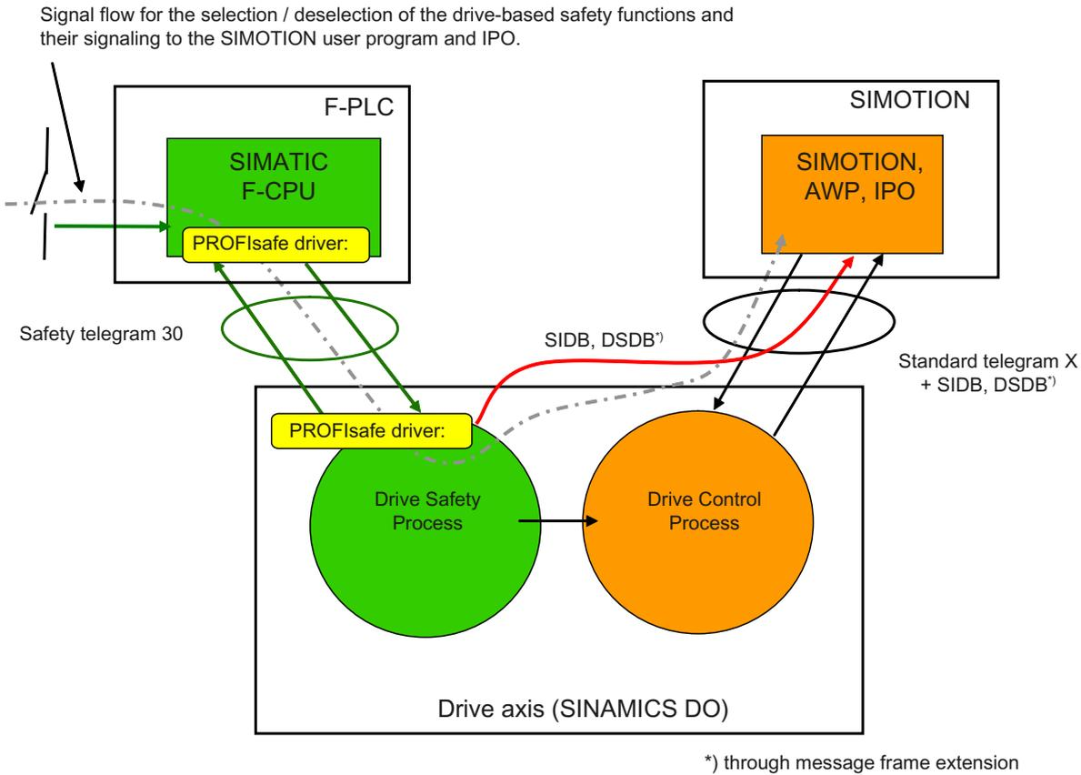
Figure 9-2 Messages and signals in drive-based safety
