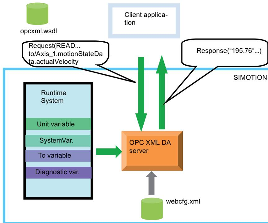
Figure 8-3 Access to the OPC XML DA server
