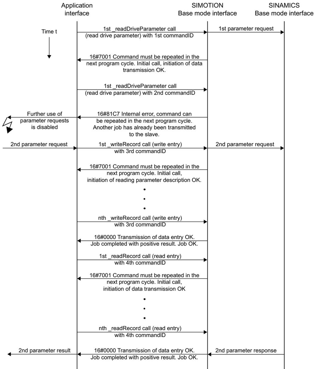
Figure 10-16 Mixed use of `_readDrive...` and `_read/_writeRecord`
