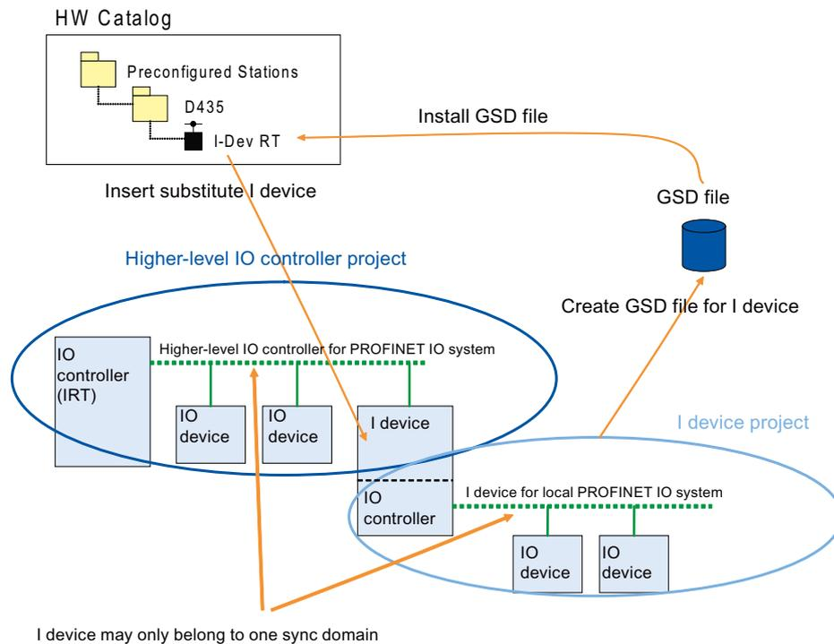
Figure 5-62 I-device configuration
