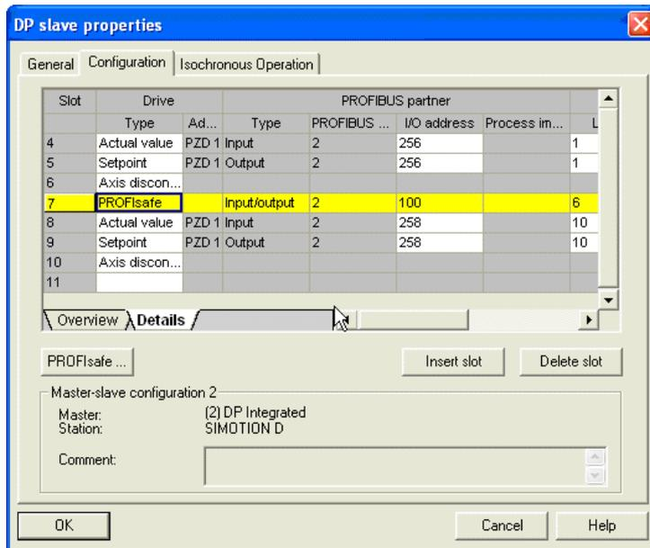
Figure 9-47 PROFIsafe configuration for SINAMICS drive unit
