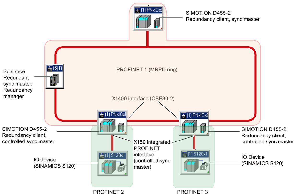
Figure 5-24 Example configuration for controlled sync master
