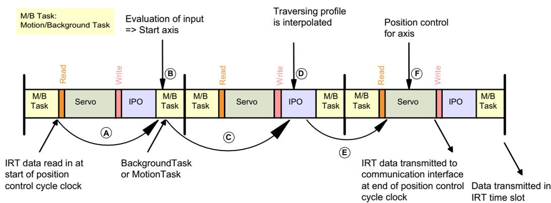
Figure 5-11 Logic evaluation for an axis in the BackgroundTask or MotionTask
