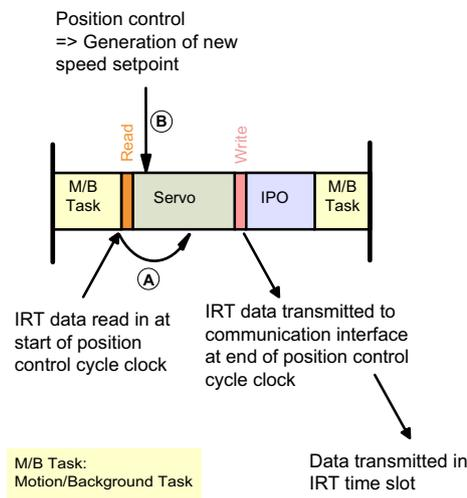
Figure 5-15 Position control time response with ServoSynchronousTask
