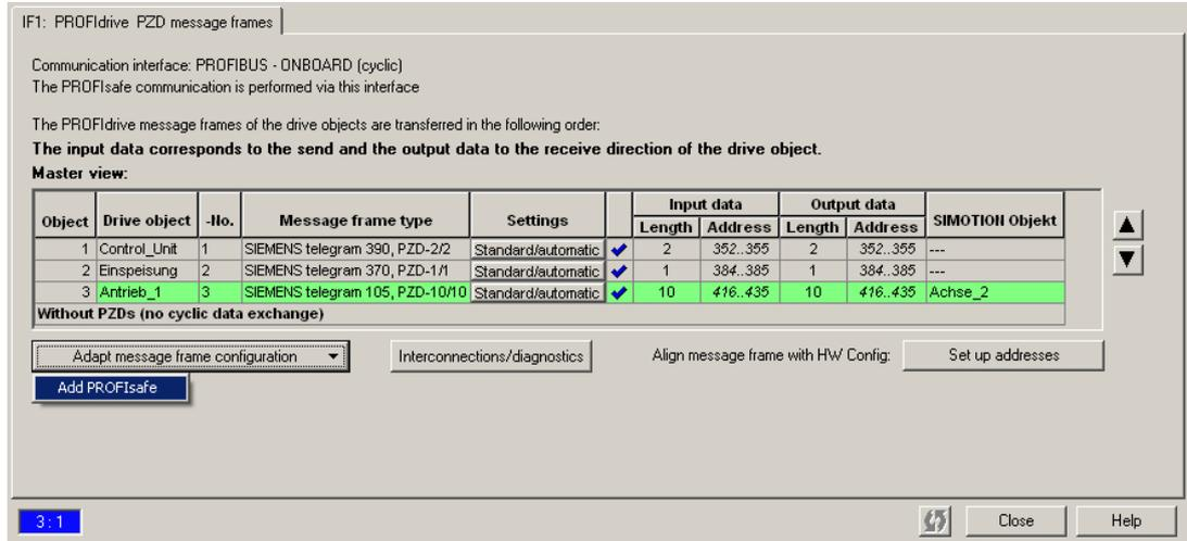
Figure 9-43 Inserting a PROFIsafe slot
