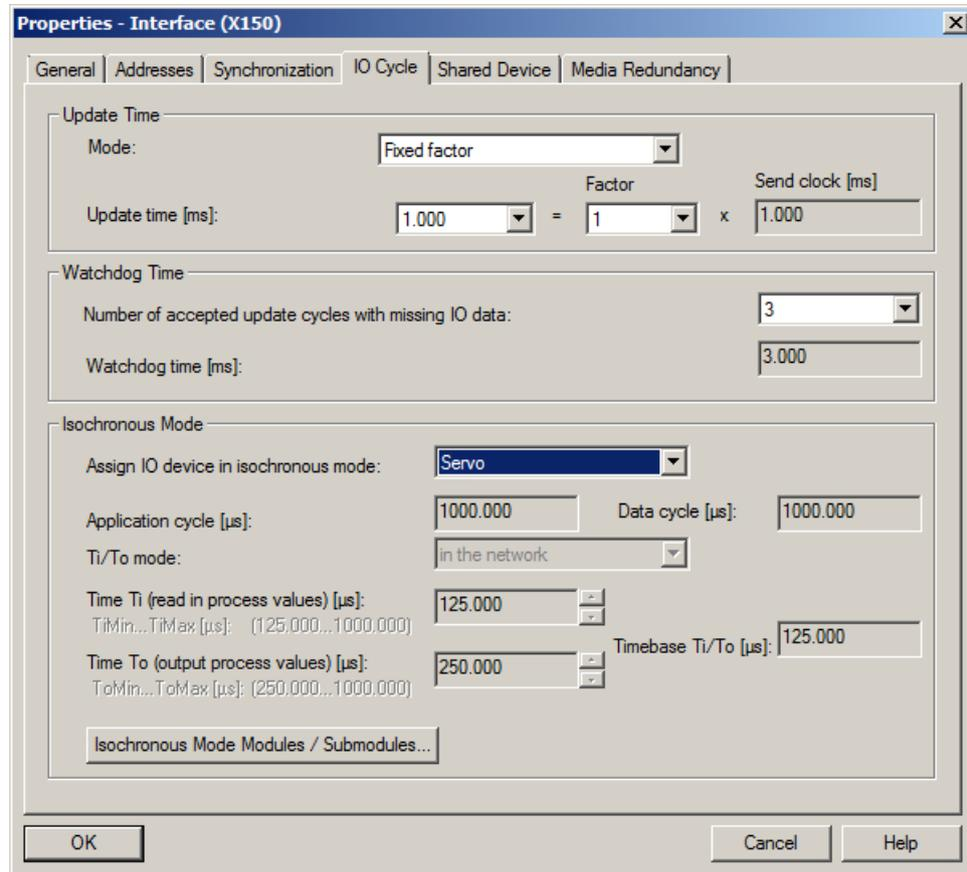
Figure 9-41 Configuring the iDevice as a slave IO device
