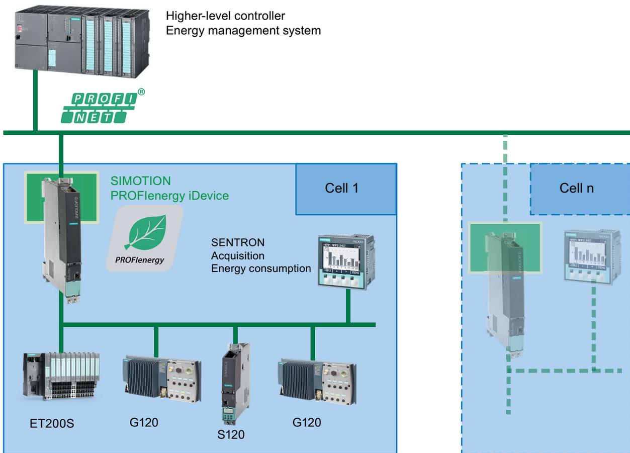
Figure 5-73 Schematic representation of the PROFenergy cell concept
