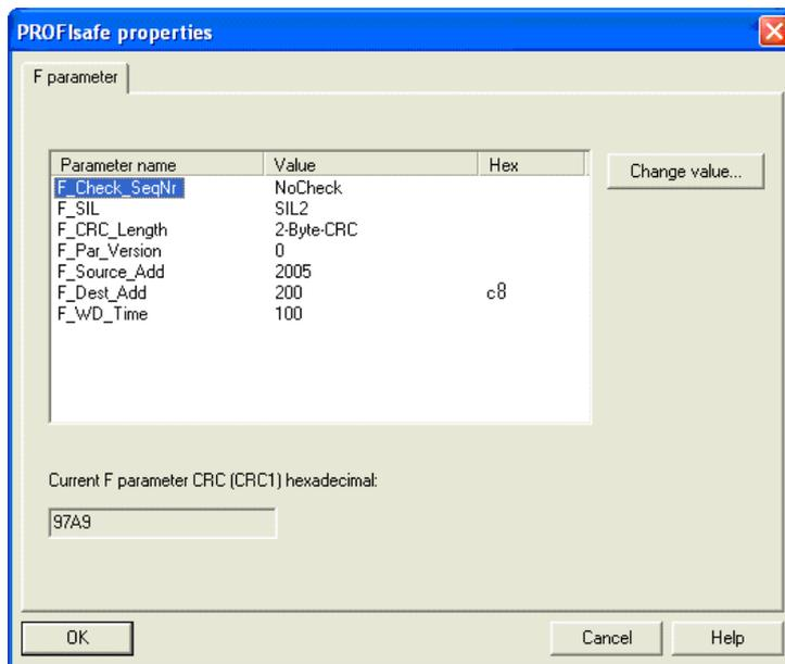
Figure 9-48 PROFIsafe properties (F-parameters)
