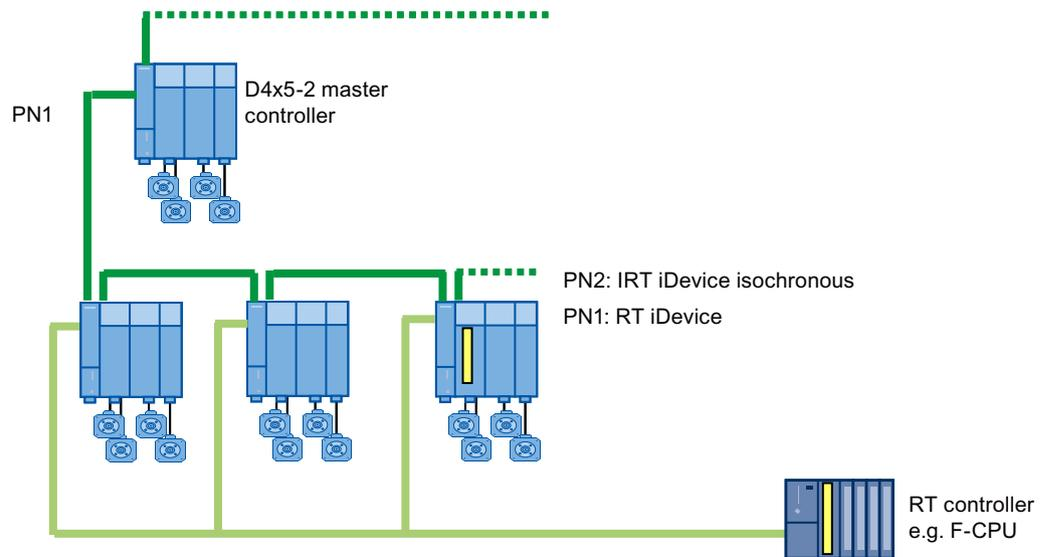
Figure 5-21 Application 5 for two PROFINET IO interfaces
