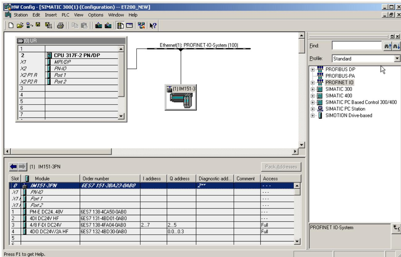
Figure 9-28 SIMATIC CPU 317F-2 PN/DP with shared device ET200S
