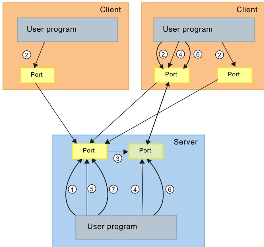
Figure 6-2 Schematic diagram showing TCP communication sequence
