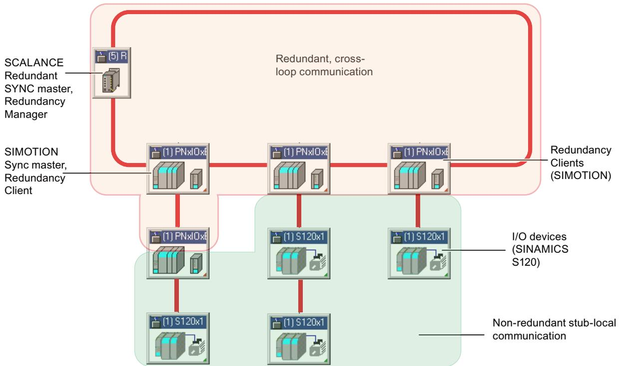
Figure 5-30 Ring configuration with SCALANCE and SIMOTION
