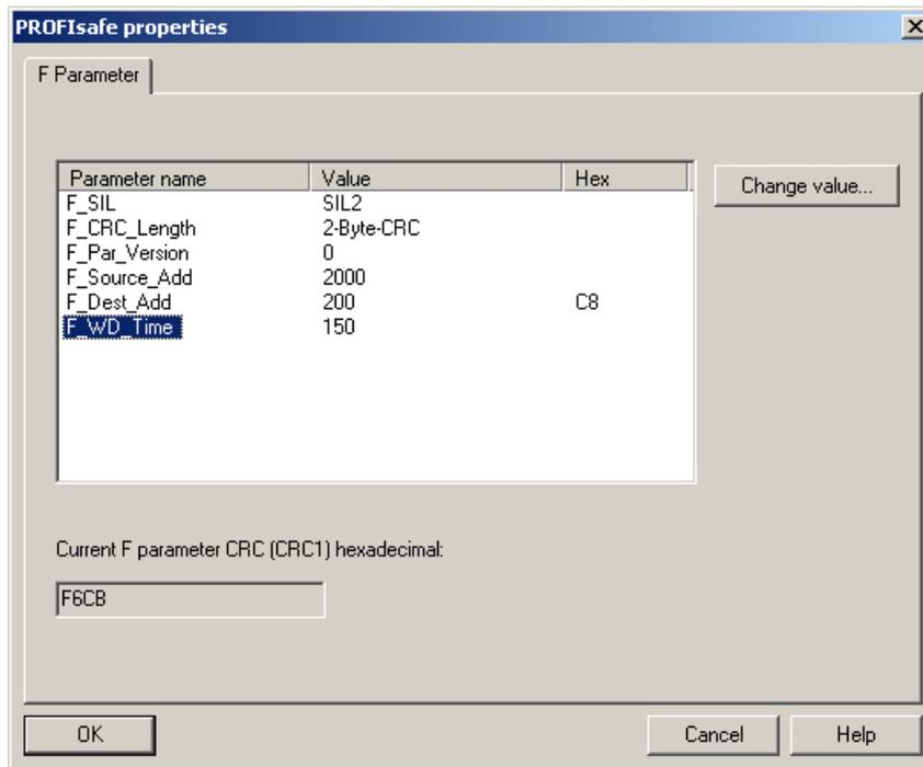
Figure 9-53 PROFIsafe properties failsafe data exchange broadcast mode V1
