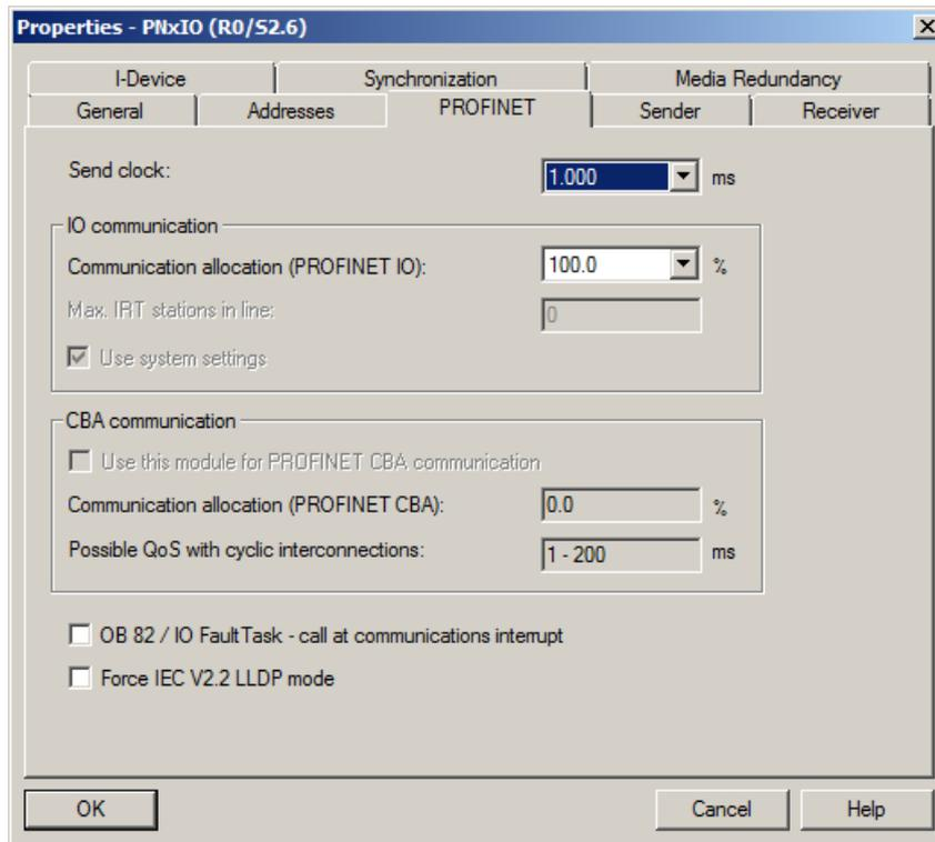
Figure 5-44 Configuring a send clock for PROFINET RT
