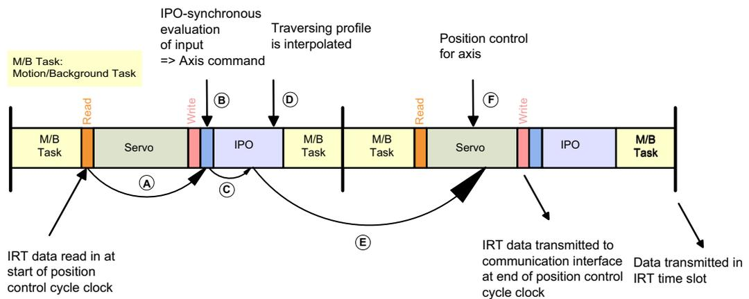
Figure 5-12 Logic evaluation for an axis in the IPOSynchronousTask
