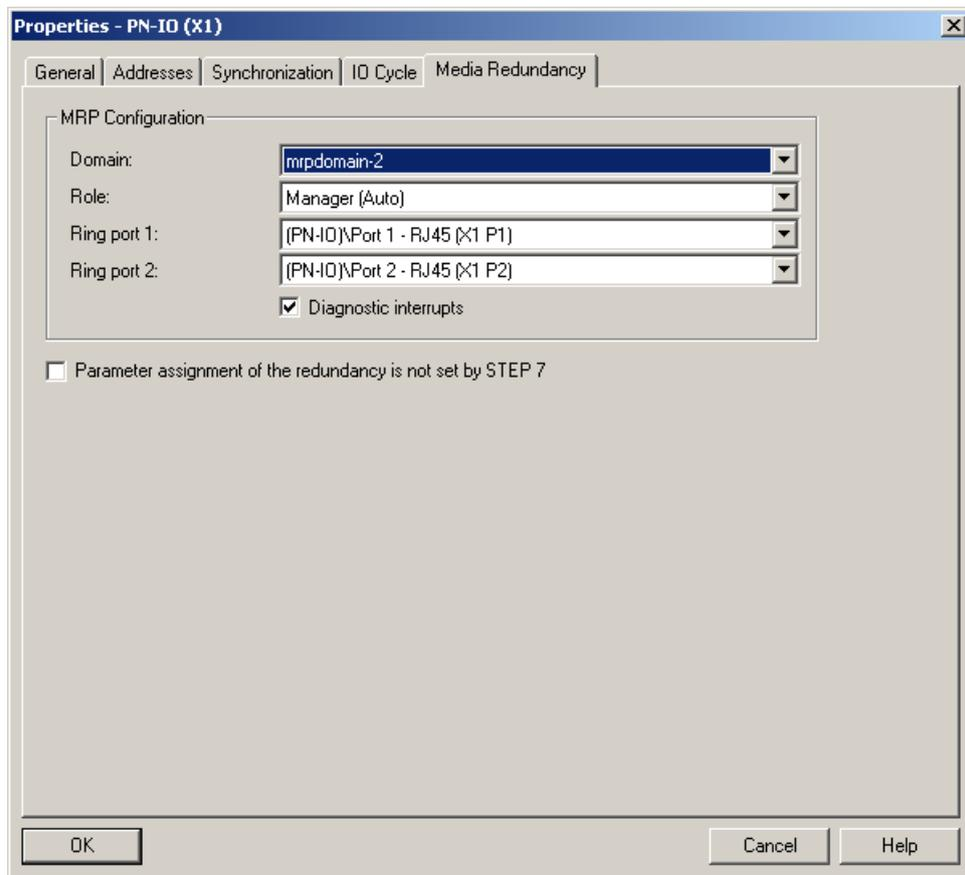
Figure 5-60 Properties Redundancy Manager
