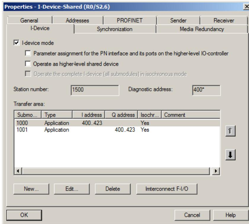
Figure 5-63 I-device properties dialog box
