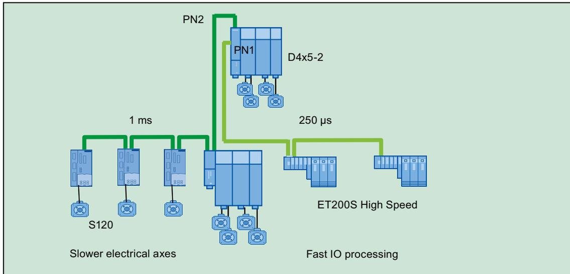
Figure 5-18 Application 2 for two PROFINET IO interfaces
