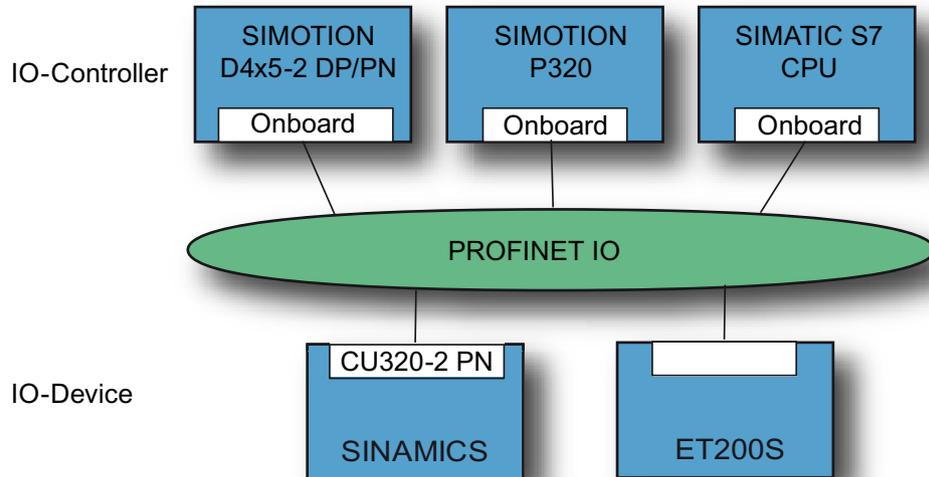
Figure 5-1 PROFINET overview IO Controller - IO Device
