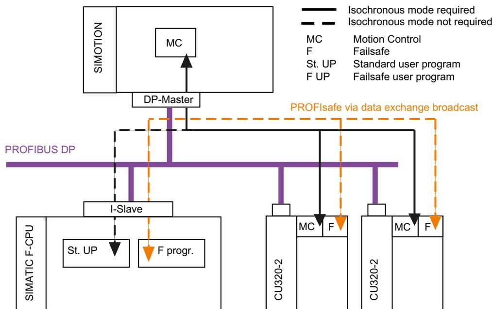
Figure 9-49 Topology of failsafe data exchange broadcast for PROFIBUS drive units
