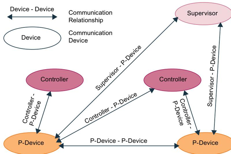
Figure 10-1 Communication between device classes according to PROFdrive
