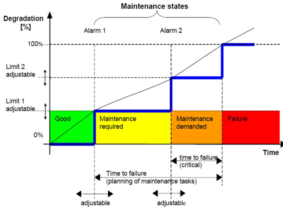
Figure 5-71 PROFINET IO maintenance state model
