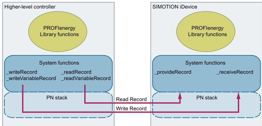
Figure 5-74 Read record and write record as iDevice
