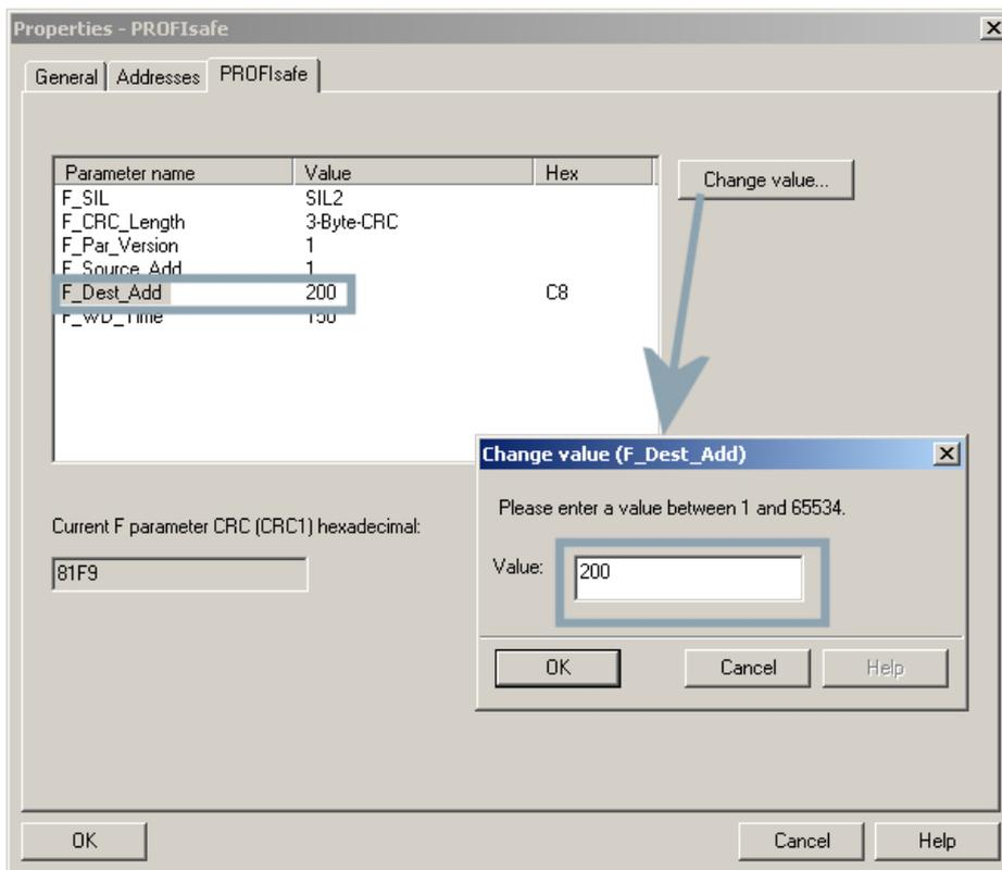
Figure 9-14 Setting the F destination address (F\_Dest\_Add)
