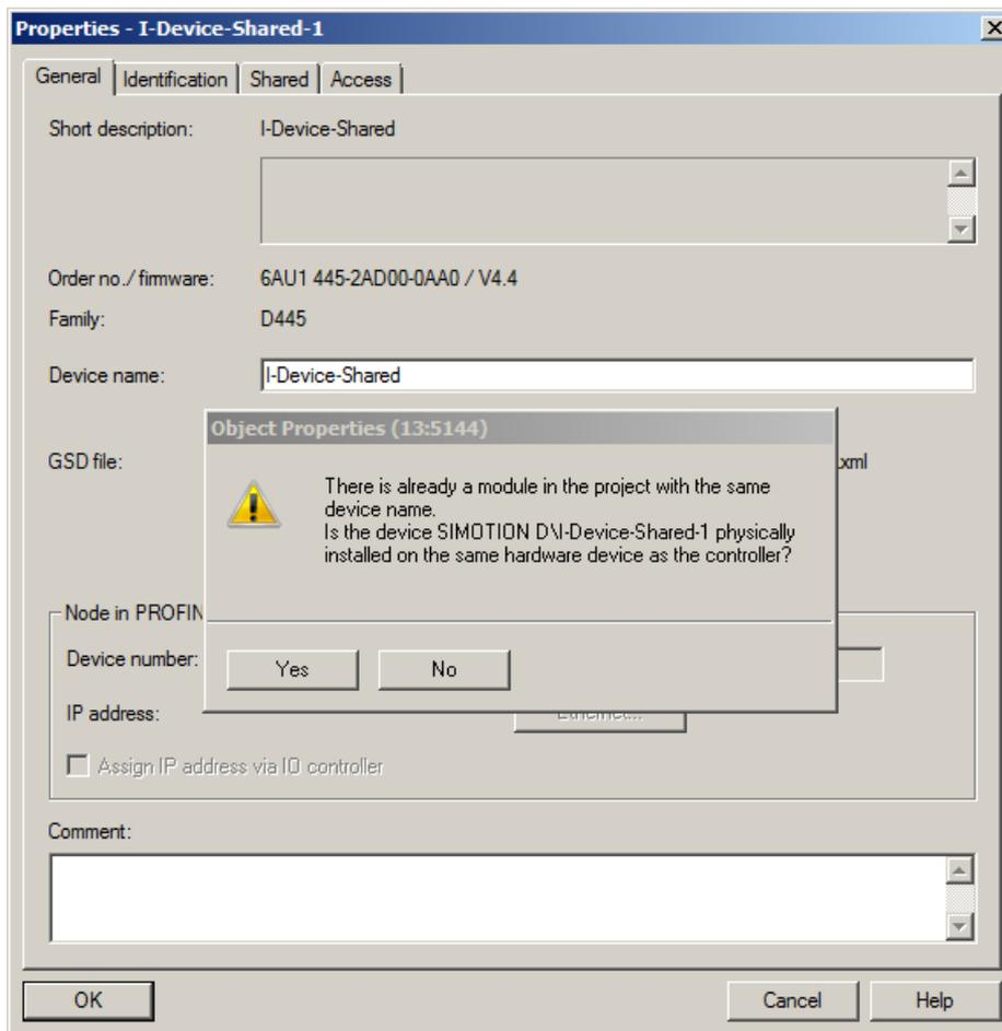
Figure 9-35 Entering a device name for the shared iDevice
