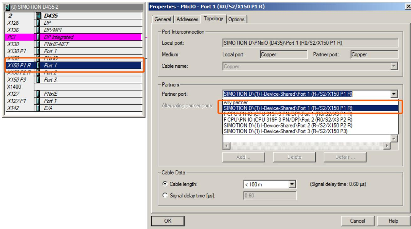
Figure 9-39 Port interconnection on the iDevice
