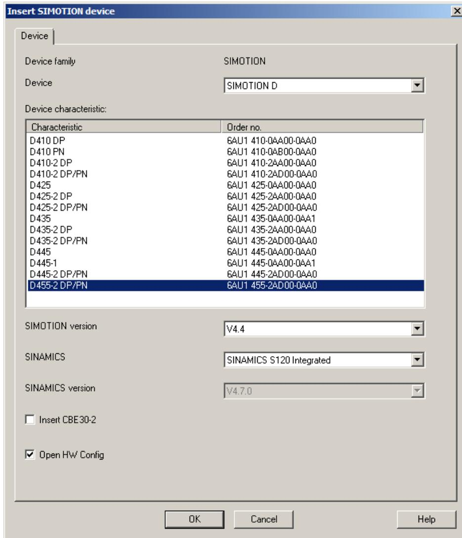
Figure 5-34 Inserting a SIMOTION device
