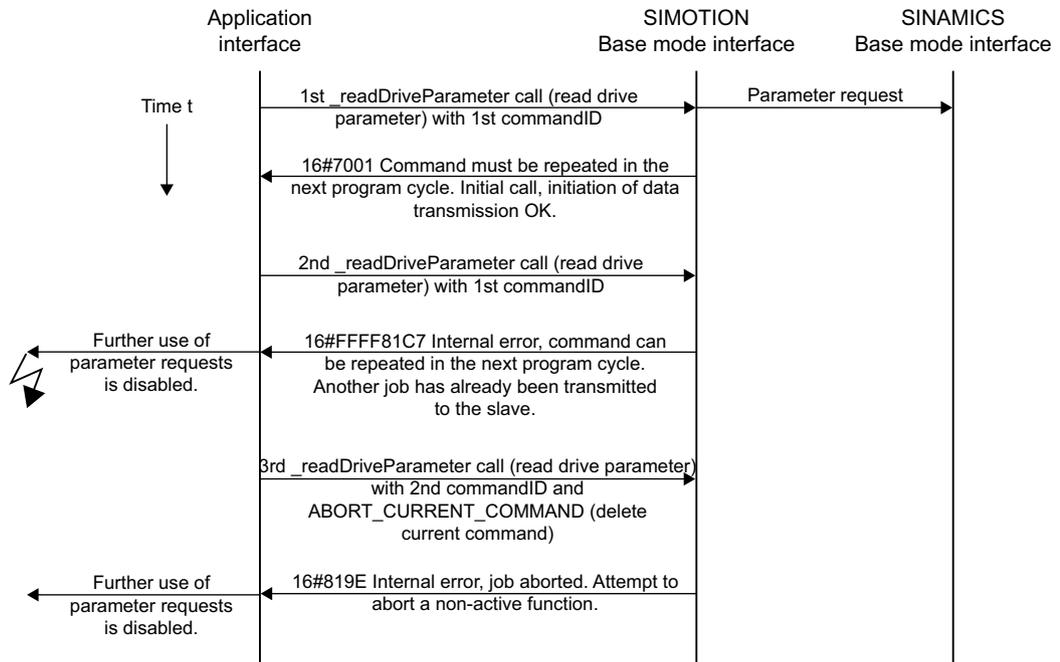
Figure 10-14 No cancellation of a \_readDriveParameter job with new CommandID
