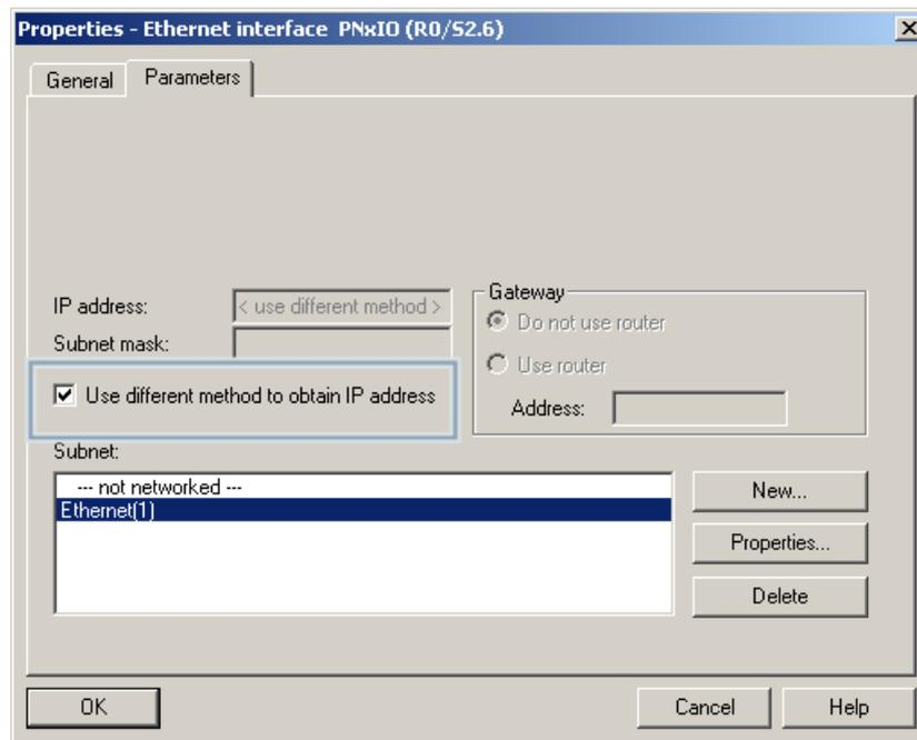
Figure 5-55 Obtaining the IP address using a different method
