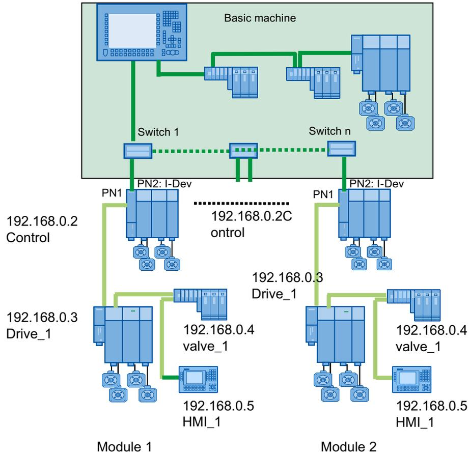
Figure 5-20 Application 4 for two PROFINET IO interfaces
