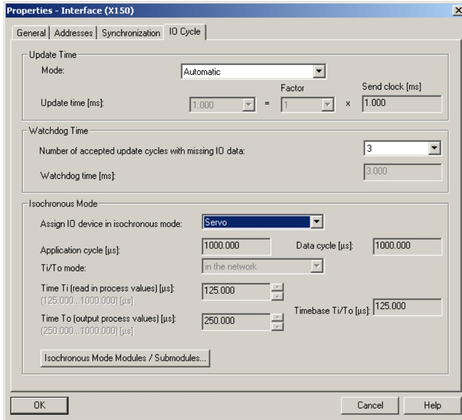
Figure 5-67 Setting isochronous mode on the I-device
