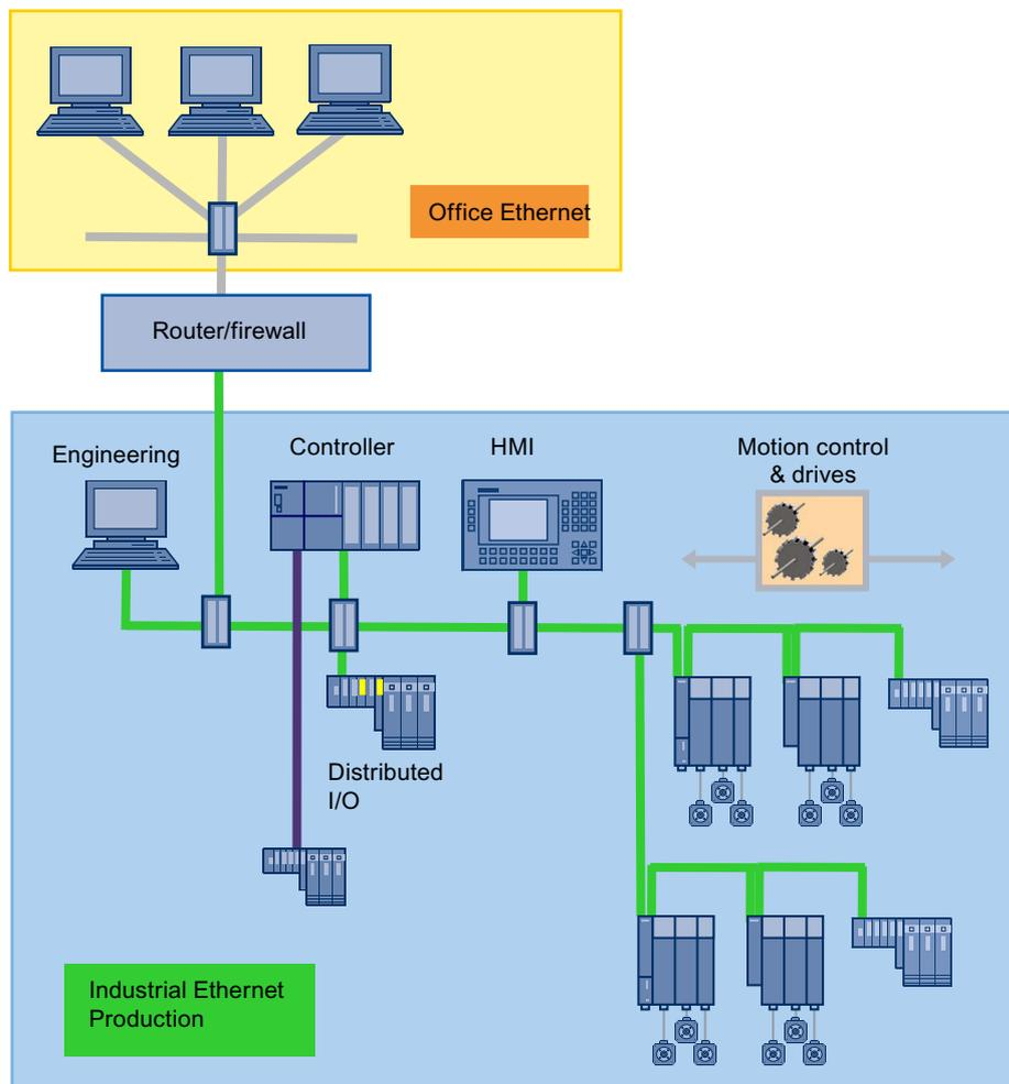
Figure 5-5 Optimized topology of a company network connection
