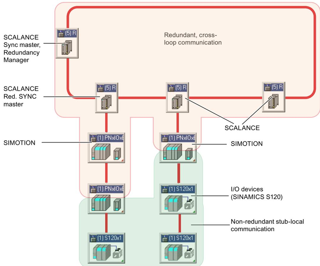
Figure 5-29 Ring configuration with SCALANCES
