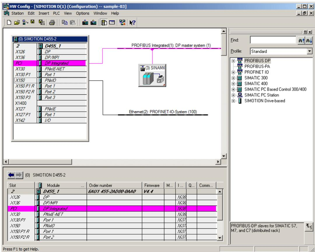
Figure 5-36 SIMOTION D455-2 DP/PN in HW Config
