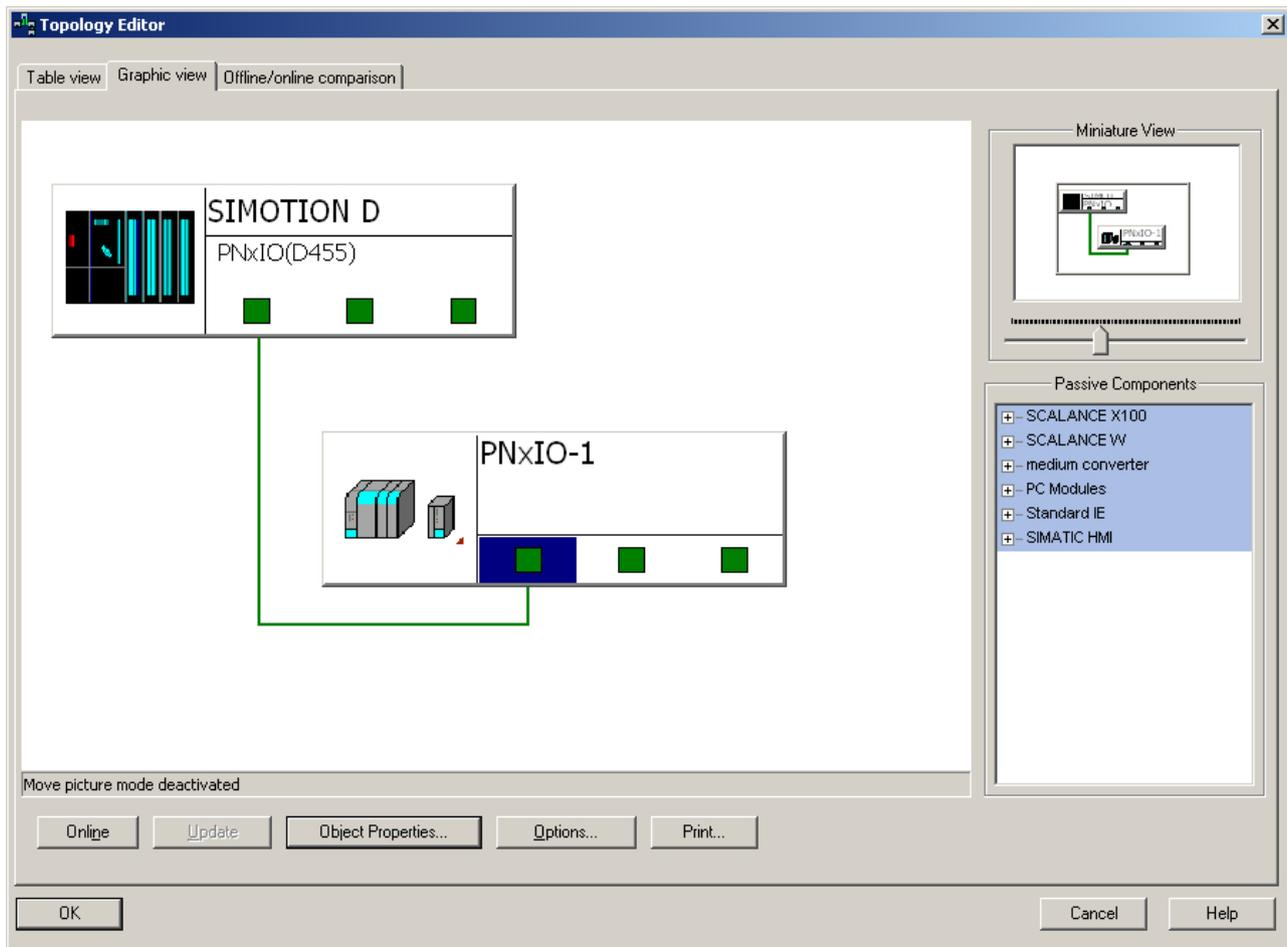
Figure 5-66 Interconnecting I-device ports
