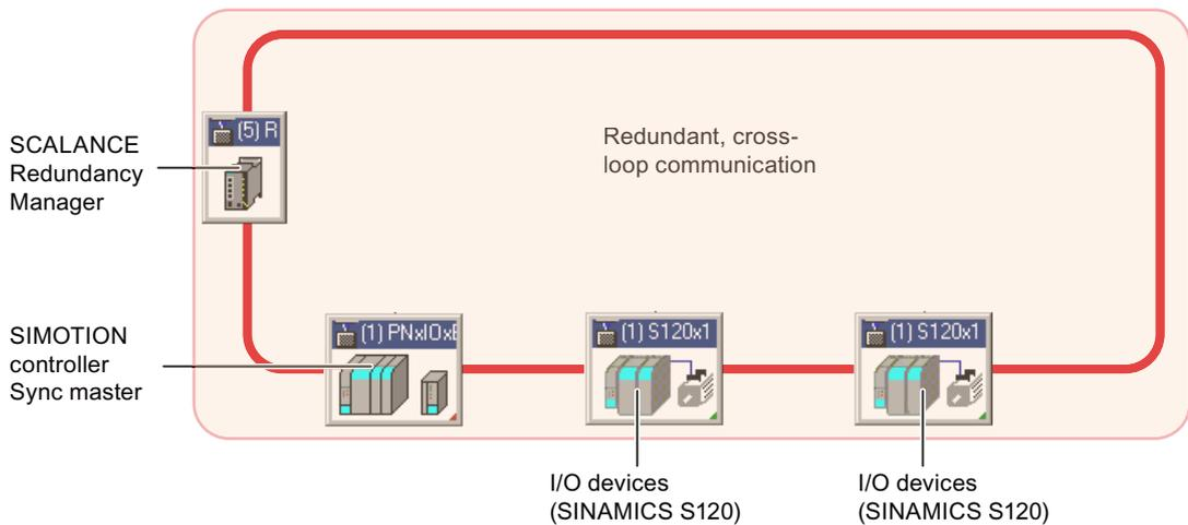
Figure 5-31 Ring configuration with SINAMICS I/O devices
