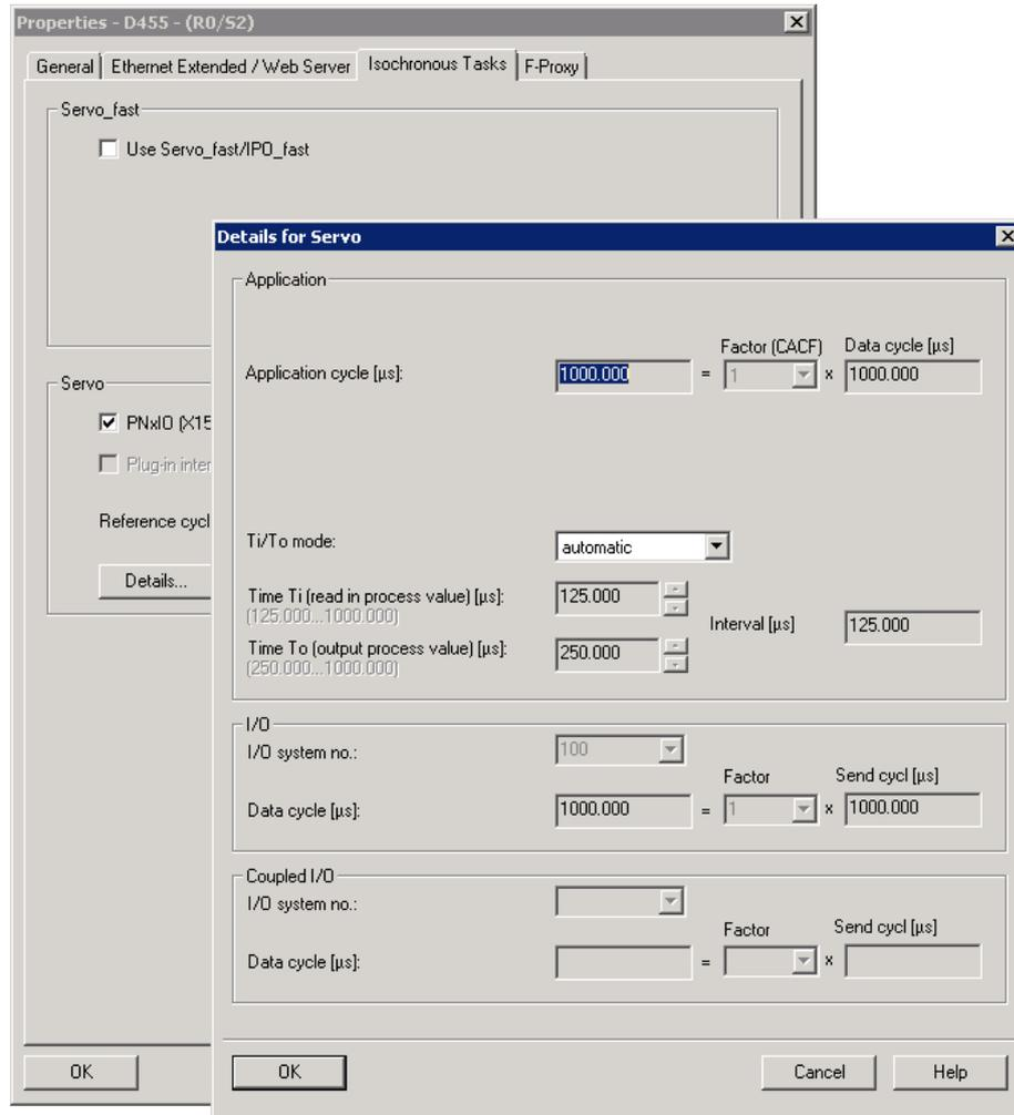
Figure 5-50 Configuring an isochronous task on the SIMOTION device.
