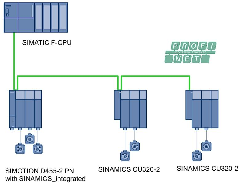
Figure 9-5 Example topology for F-CPU master with SIMOTION D and lower-level drives
