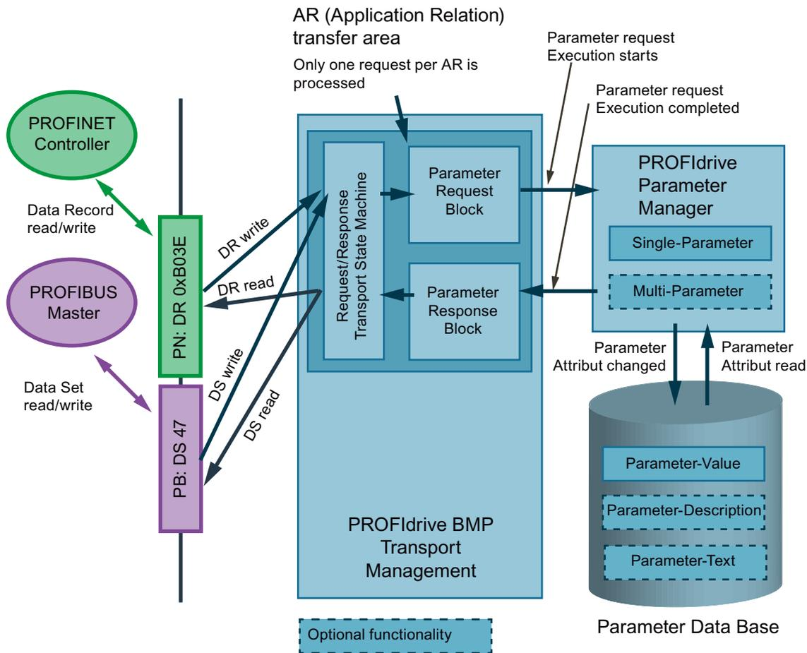
Figure 10-5 Function of the PROFdrive parameter channel
