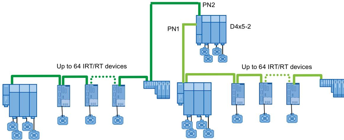
Figure 5-17 Application 1 for two PROFINET IO interfaces
