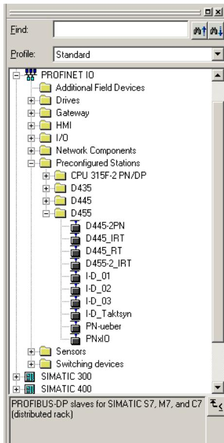
Figure 5-64 iDevice entry in the hardware catalog
