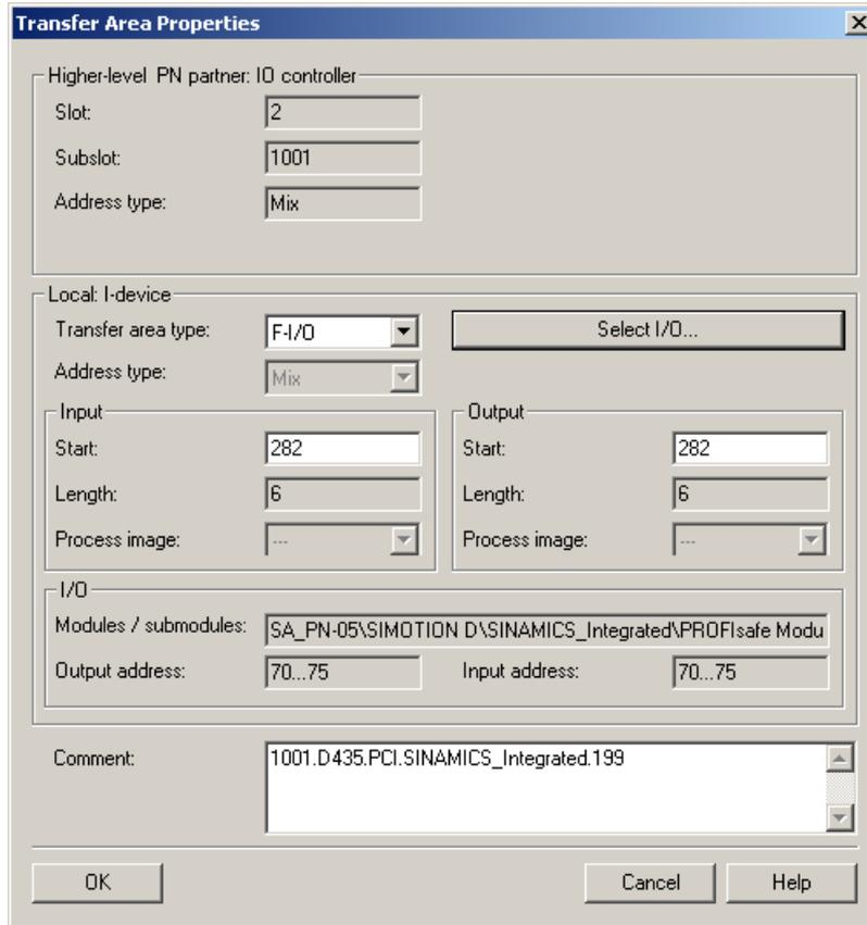
Figure 9-21 Properties of I-device transfer area, comment
