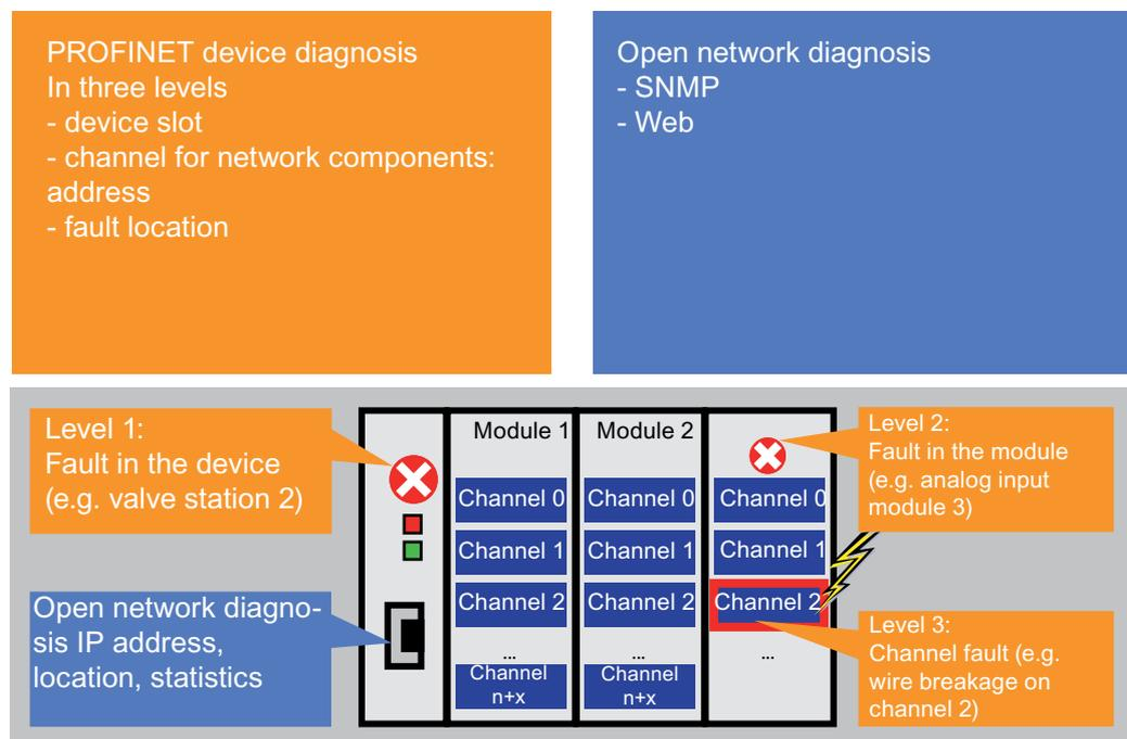
Figure 5-70 Diagnostics overview using the example of ET200
