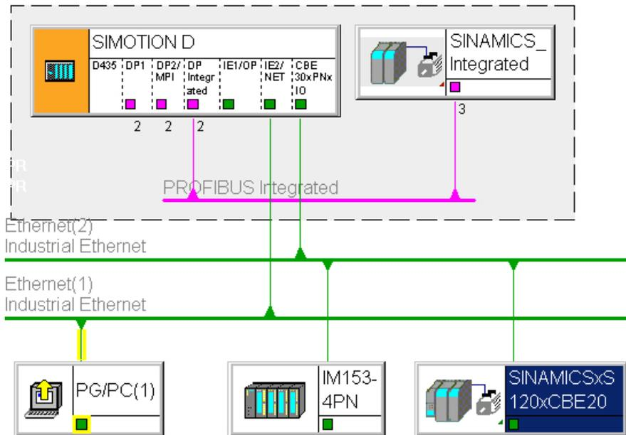
Figure 7-4 Example for PG/PC to Ethernet X120, X130
