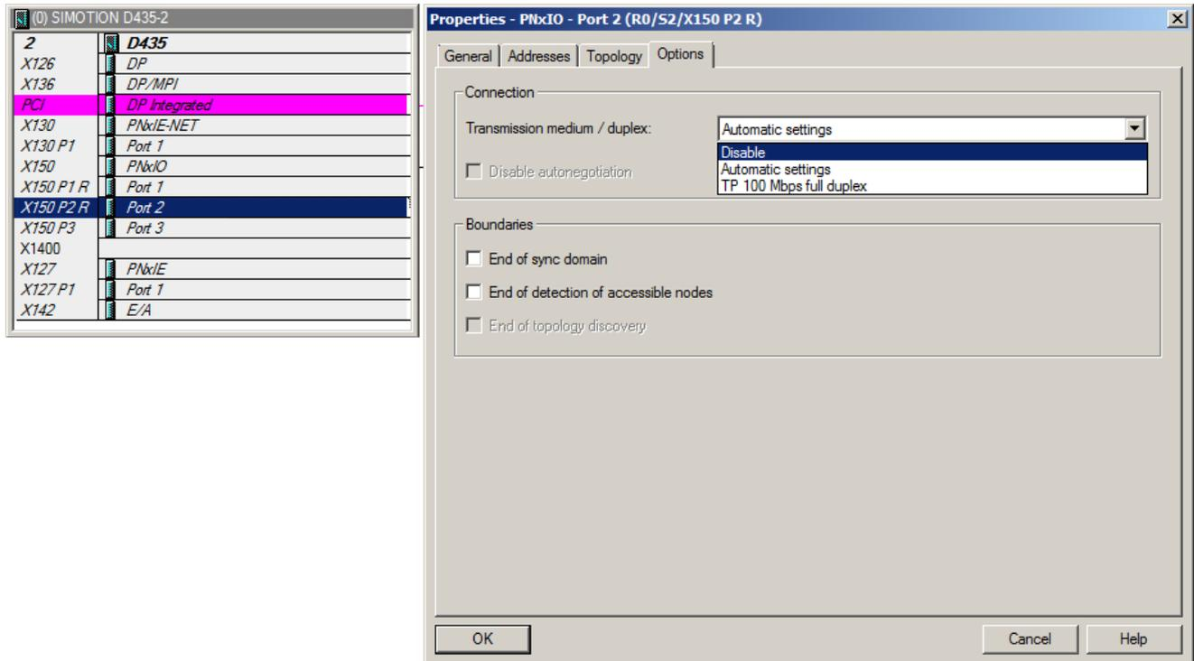
Figure 6-5 Deactivating PN ports on SIMOTION CPUs
