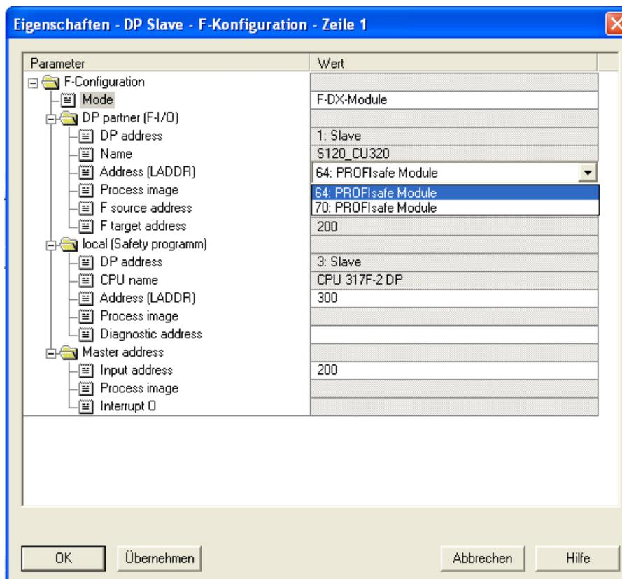
Figure 9-51 Properties of failsafe configuration for data exchange broadcast
