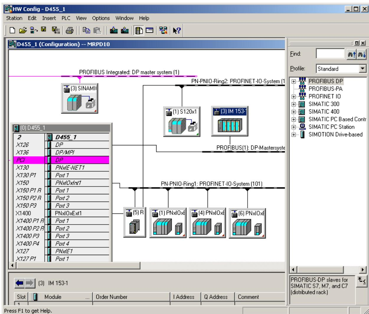
Figure 5-56 Ring project in HW Config
