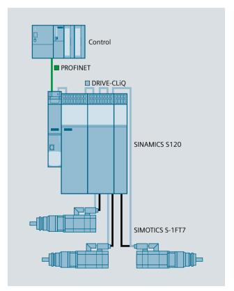
Integrating the SIMOTICS S-1FT7 motor into the SINAMICS S120 drive system
