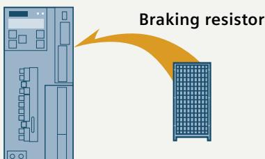
All frame sizes have an integrated braking resistor to dissipate the regenerative power for fast braking.
