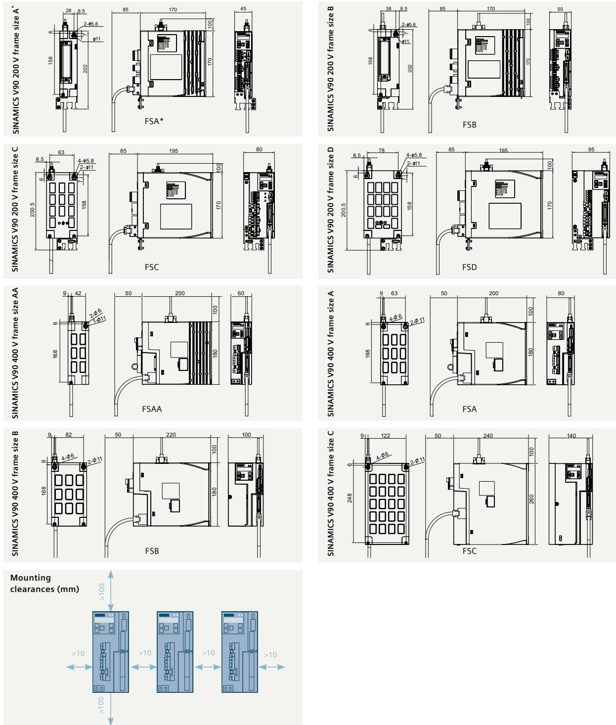
\* SINAMICS V90 PROFINET 200 V version is not available in frame size A (FSA).
