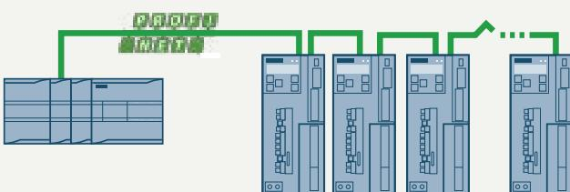
SINAMICS V90 PROFINET version features a PROFINET interface, enabling real-time transmission of user/process data and diagnostic data with a single cable.
