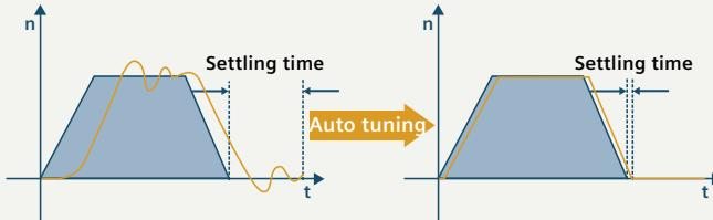
Control loop parameters are optimized automatically. One-button tuning can be used when commissioning. This allows machines to achieve a high dynamic performance and smooth operation in a wide range of applications.
