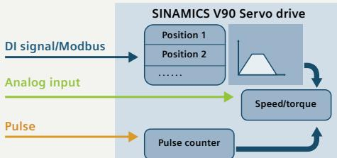
Pulse train input position control mode (PTI), internal position control mode (IPos) with traversing block or Modbus, speed control mode and torque control are all integrated in the SINAMICS V90.
