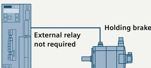
Integrated holding brake switch – the brake can be directly connected to the drive when a motor with holding brake is used.
