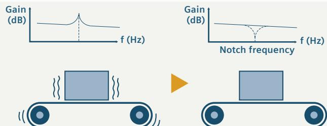
When this function is activated the drive identifies mechanical resonance frequencies and automatically suppresses these using a filter. Vibration and noise during operation are reduced.
