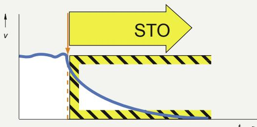
The STO function is a standard feature of all SINAMICS V90 servo drives. This function prevents the motor from moving unexpectedly and complies with safety standard SIL 2 according to EN 61508 resp. PL d, Cat 3 according to EN ISO 13849. This safety functionality can be realized without additional components (activation only via terminals of SINAMICS V90, not supported via PROFINET/PROFIsafe).
