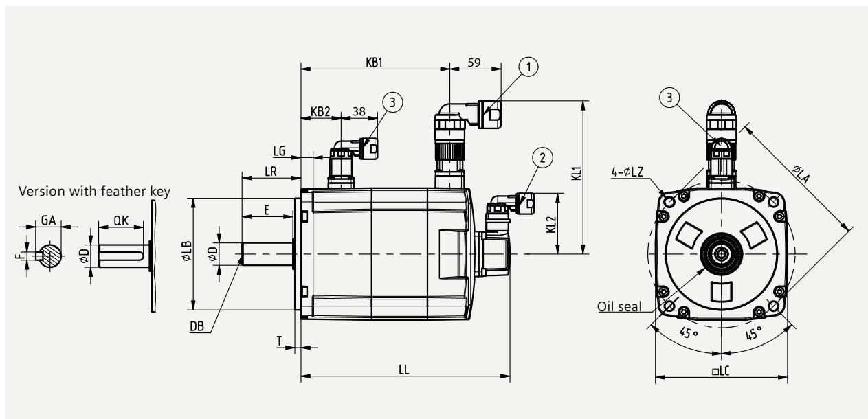
Note: ① Power connector, ② Absolute encoder connector, ③ Brake connector
