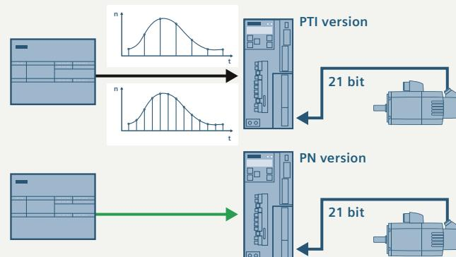
The encoder is available up to 21-bit resolution (approx. 2.1 billion pulses per motor rotation).
