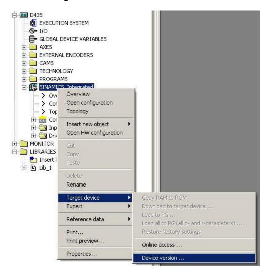
3. The Device version dialog window will open. It lists all devices with the appropriate firmware versions. Select the required firmware version and close the dialog window.
