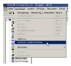
6. When opening the "The associated symbolics could not be found" dialog (as shown in the examples below), the source names must be replaced. The correct notation for the names must be taken from the user project. The cause for this procedure is a subsequent change of the unit name syntax (uppercase/lowercase) in the Simotion project by the user. If this window does not open, all variables have been found and reconnected.
