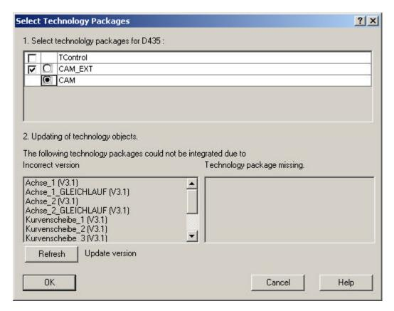
Activate the technology packages checkbox. Because the technology packages must have the same version as the kernel, the same version as the kernel is automatically assigned to each technology package in the SIMOTION SCOUT as of V3.0.
