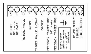
The supply voltage should be connected to terminals 11...12 as indicated in the connection diagram on the housing cover.
