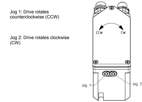
Holding both keys simultaneously for longer than 500 ms sets the actual drive position to 0.
