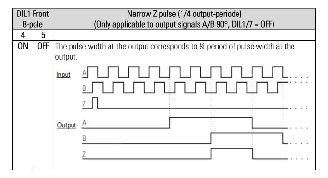
In this operation mode, only division ratios may be used, which together with the A/B divisor deliver clear and completely results. A division with rest causes that the Z pulse at the output can fluctuate around an input or output period.
