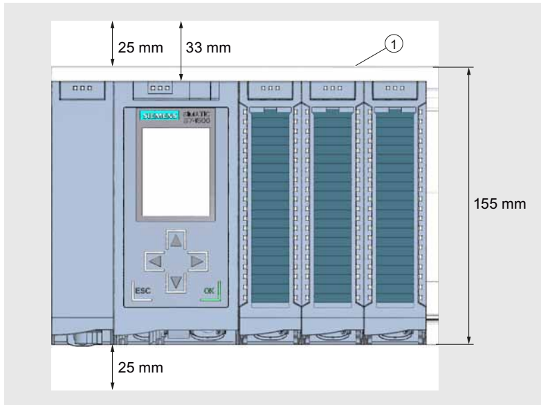
Figure 5-1 Minimum clearances in the control cabinet
