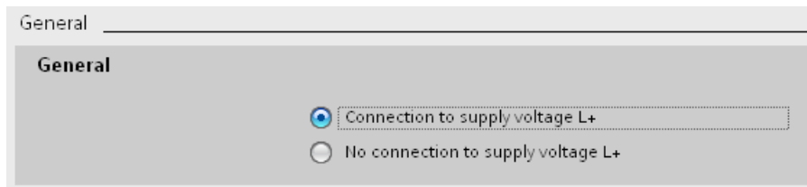
Figure 4-5 Supply voltage via the CPU and system power supply
