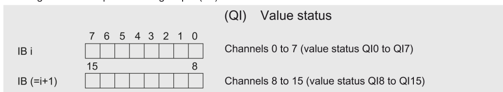
Figure 4-1 Address space for configuration as 16-channel DQ 16x24VDC/0.5A ST with value status
