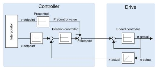
The MC-Interpolator [OB92] calculates the setpoint position for the axis. The difference between the setpoint and actual position is multiplied by the value of the position controller. The resulting value is added to the precontrol value and output as setpoint speed at the drive.
