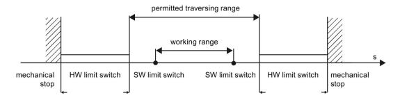
Hardware limit switches are limit switches that limit the maximum "permitted traversing range" of the axis. Hardware limit switches are physical switching elements that must be connected to interrupt-capable inputs of the CPU.
