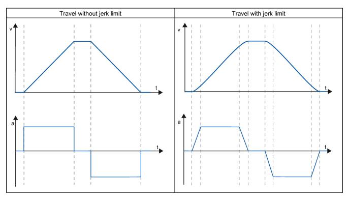
The jerk limit gives a "smoothed" velocity profile of the axis motion. This ensures, for example, soft starting and braking of a conveyor belt.
